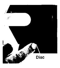
For very thin stamps turn to the right (clockwise). For very thick stamps turn to the left (counterclockwise). Push handle back in, until engaged. Re-tighten screw.
